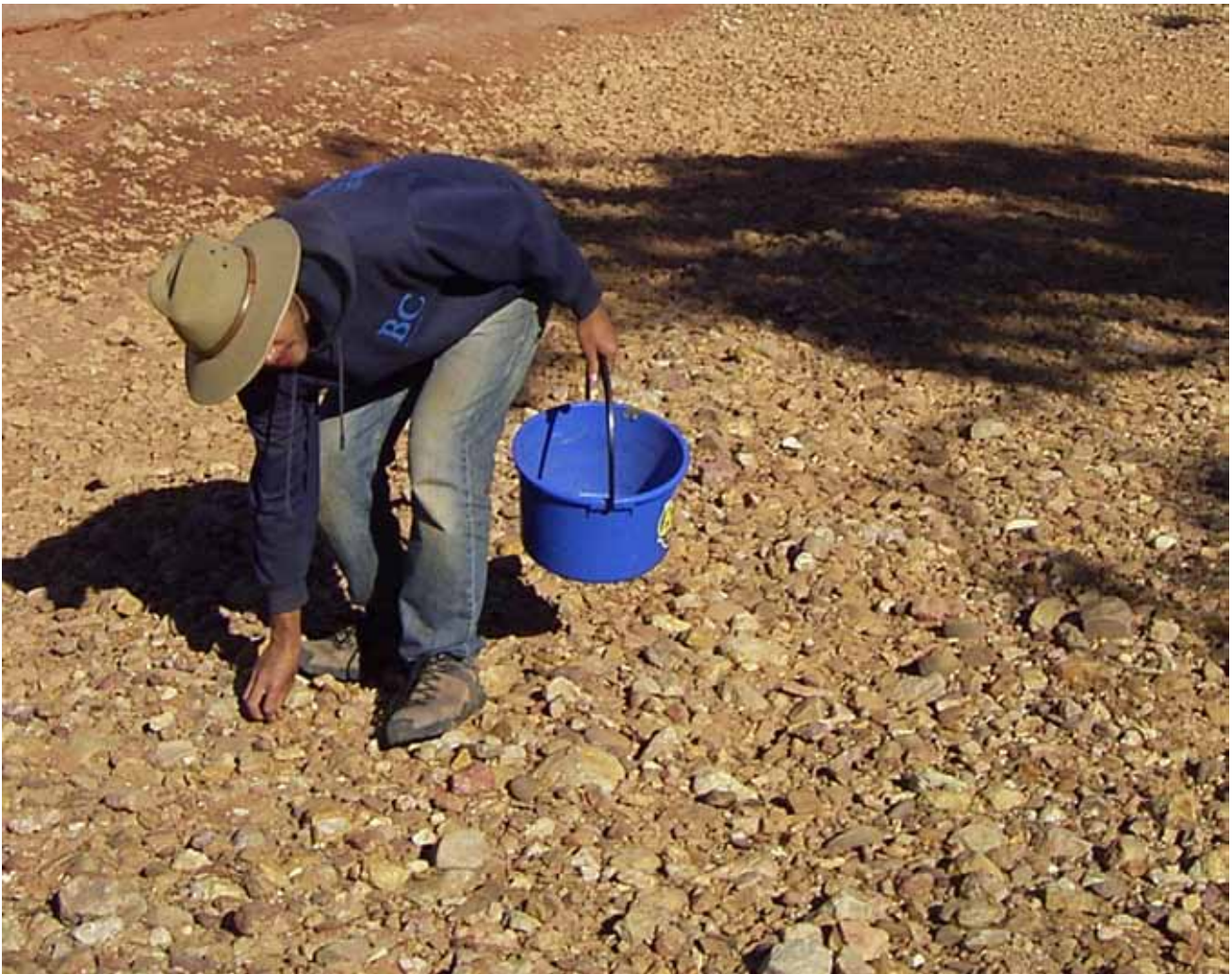
Figure 2. Sample selection for the Wolman pebble count as applied in this study. Note that samples are collected with eyes averted to avoid sampling bias.
