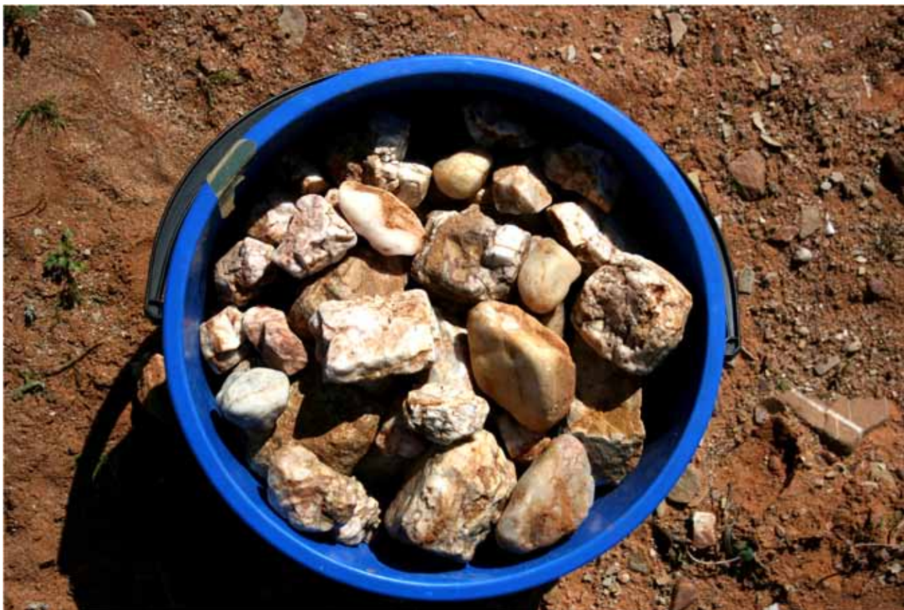
Figure 5. Quartz cobbles collected during the application of the Wolman Method. Quartz cobbles found in creek beds and in desert pavements have a smooth, rounded cortical exterior.
