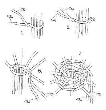
The handles of bags from the Moreton region were made of three strand plaits, using thin strips from the leaf of the pandanus. The leaf was usually dried in the sun to make it firmer, but to save time it could also be heated over a fire for a few minutes.
