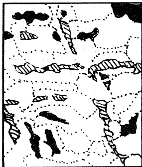
Fig. 1.—Small portion of the etched surface showing the breaking up of the taenite bands by granulation, which has already affected the kamacite bands. The hatched portion is taenite, the black portions are inclusions, and the dotted lines indicate the boundaries of the grains.
